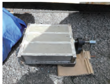
When collecting a paste specimen of SKY-G1/SKY-CSP60% (W/C). With normal cement, bleeding occurs immediately after collection and the cement paste settles.
