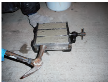
When collecting a paste specimen of SKY-G1/SKY-CSP60% (W/C). With normal cement, bleeding occurs immediately after collection and the cement paste settles.
