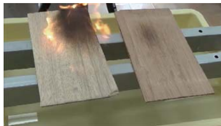
Left side: untreated - right side: flame retardant treatment
