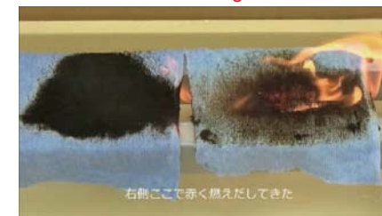
Left side: Flame retardant treatment - Right side: Not processed
