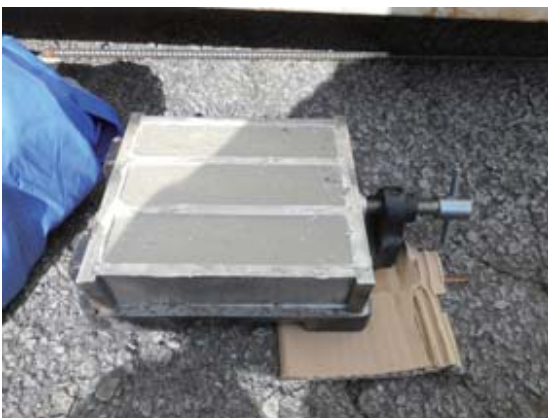
SKY-G1, SKY-CSP 60% (W/C) paste Specimen 1 day passed. Usually cement paste bleaches and precipitates, but bleaching water does not rise and it solidifies.
