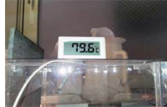
Untreated plate: irradiation test plate back temperature
