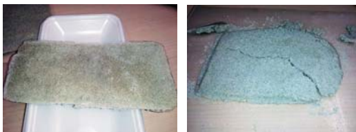
When it was sprayed on silica sand No. 5 and it solidified, it got soft and it sucked in water even if it solidified
