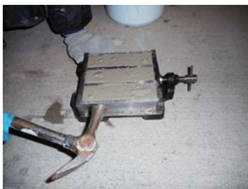
SKY -G1/SKY-CSP 60% paste specimen collection. In ordinary cement, surplus water after mixing is floated immediately after collection, and the cement paste sediments.
