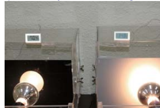
Measurement of irradiation temperature by 100 W Ref Light bulb
