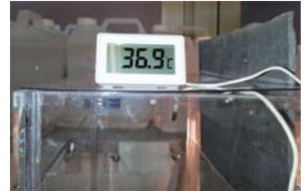
Irradiation test plate backside temperature
