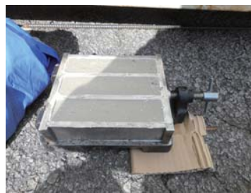
SKY-G1 / SKY-CSP 60% paste Specimen 1 day passed. There is no floating of the surplus water, and it does not stretch but solidifies.
