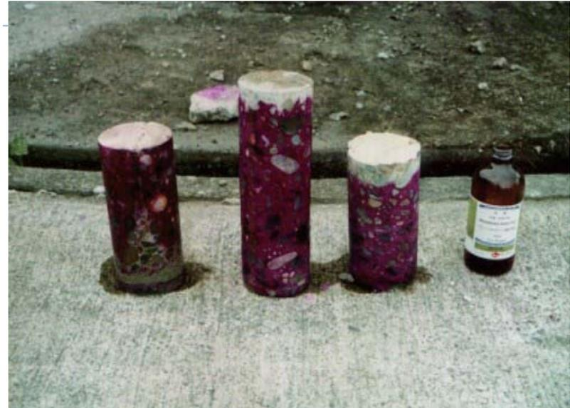
Check the position of the internally arranged reinforcement and fix the core drill before construction. While sending water, open the core.
