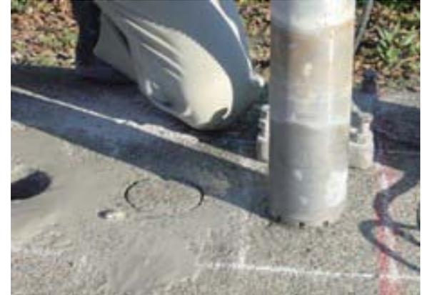
A wire is wrapped around the cut concrete, and the part there is cut off by hitting a tagger. If raising it slowly and testing at the building material center, wrap it immediately and prevent oxidation. Normally, a phenolphthalein solution is applied on the spot to see the reaction.
